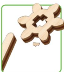
**ENG** Clean the burrs on the parts using the universal "Helper" (H) instrument.
